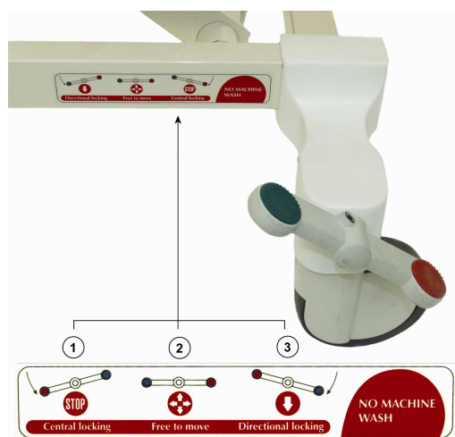
Figure 3. Locking of the central locking castors
