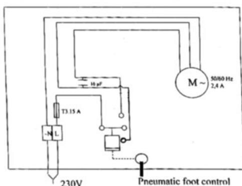
**Figure 12: Circuit diagram of Delta tables**
